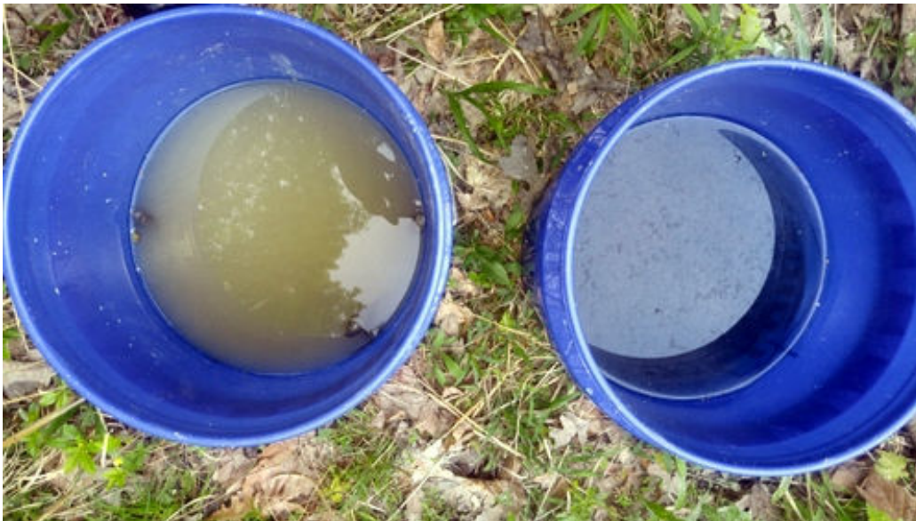
A 4-inch square piece of bentonite liner material was placed in the bucket on the left (notice the dead green frog larvae floating on the surface after 24-hours). The bucket on the right does not contain the bentonite liner material.
